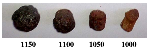
Fig. 8 the shape of pellets change with temp.
